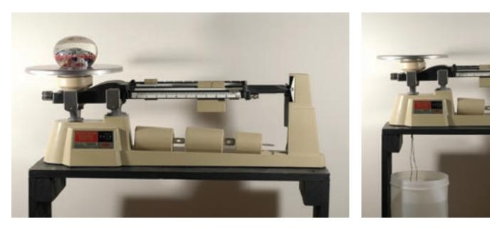
Weighing paperweight in air (left) and while submerged in distilled water (right)
